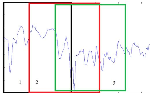
Figure 2.3: Figure illustrating windowing operation
