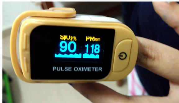
Figure 2.1: Pulse oximeter was used for obtaining ground truth heart rate. Pulse oximeter provides heart rate in Beats Per Minute (BPM) as well as oxygen saturation level
