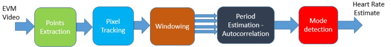
Figure 2.5: Block diagram - Mode based estimation
