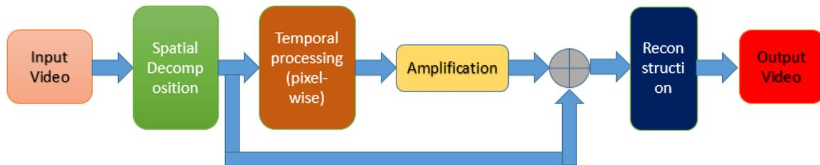
Figure 1.1: Block diagram of EVM Framework
