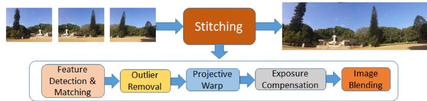
Figure 1: Pipeline of Stitching Algorithm
